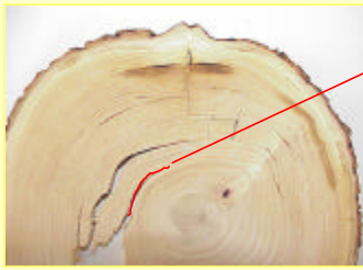
Fig. 1: Example of a ring shaken chestnut disc.
