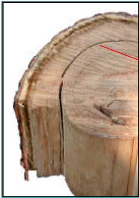
Fig. 1: Example of ring shake in chestnut wood.
