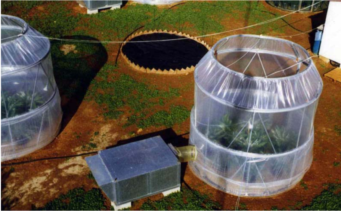
Figure 6. CEAM-UMH Open Top Chamber facility in Benifaió. Different species of plants were fumigated with enhanced ozone levels in order to induce visible injury in their leaves.
