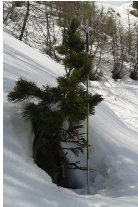
Figure 2.2: Field investigation: Example of measuring the tree height and snow depth, perpendicularly underneath the tree tip
