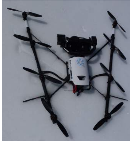
Figure 2.1: The UAS: The AscTec Falcon 8 with the Sony NEX-7 camera (©Yves Bühler)
