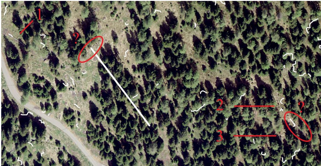
Figure 11: The fine white lines represent the R-Studio product which was derived through vectorization.
