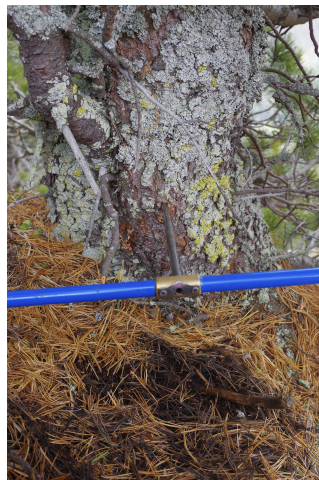
Figure 4: Increment borer for age estimation of pine
