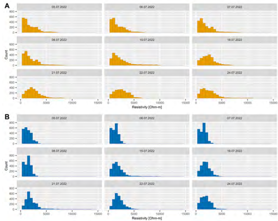
Figure 66: Histogram of the modelled electrical resistivity values of the Wenner-Schlumberger array during July survey.
