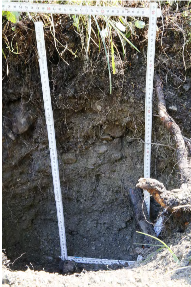
Figure 53: Soil profile at Well001 with depth of 60 cm. The soil profile was done during the installation of the sensor and data loggers.
