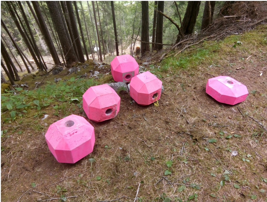
Figure 2.2: Four EOTA 111 45kg and one EOTA 221 45kg test block. ©A. Caviezel
