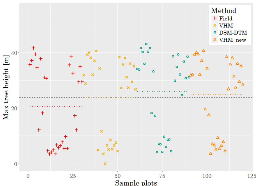
Figure 21: Distribution of measured maximal heights. The total sum of squares ( SSY = 23558.14 ) as the sum of squares of the distance between each data point to overall mean (dashed grey line) and the error sum of squares ( SSE = 23078.06 ) is the sum of the squares of the distance between each data point to its particular method mean (coloured dotted lines).
