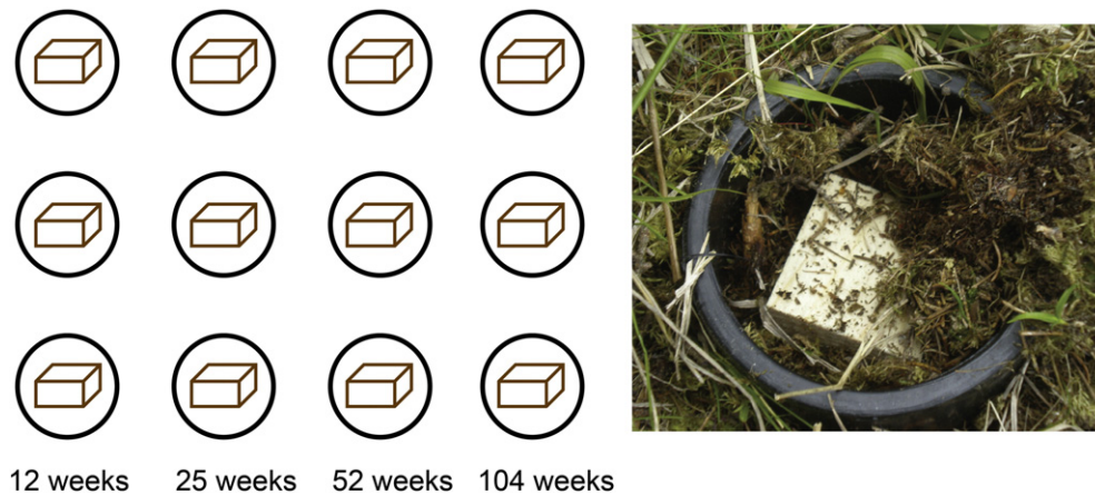
Fig. 2. Set-up of the experimental plots with wood blocks. For each time segment, three replicates were used. Wood blocks with a uniform shape and size were placed into the 'mesocosms' (i.e. open tubes inserted into the soil) on the soil surface and left for the indicated duration (weeks).
