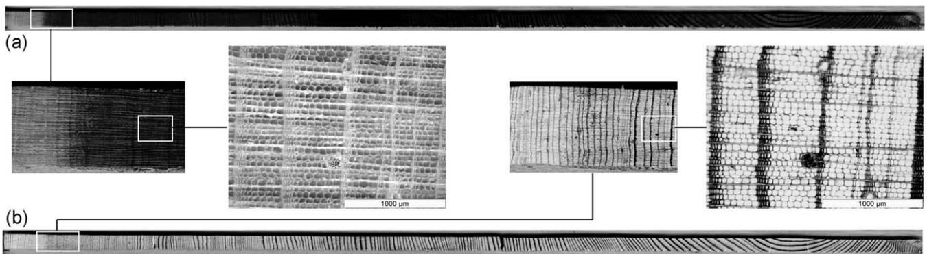
**Fig. 4.** (a) Scan image of a *Larix decidua* core surface cut by the core-microtome without further preparation. Although the rings are not very distinct at a lower magnification, the high magnification illustrates the visibility of the single cells. (b) The same core as in (a), but here the cells are filled with white chalk powder. This enhances the visibility of the ring structure even at lower magnifications.
