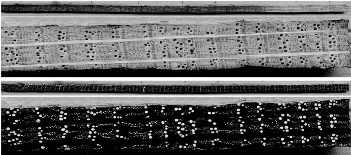
**Fig. 7.** Scan images of a *Quercus petraea* core at two different magnifications. The upper images show the core after cutting without further preparation. For the lower images, the core was stained with a black felt marker and then the cells were filled with white chalk to enhance the contrast for image analysis (compare Fig. 8).
