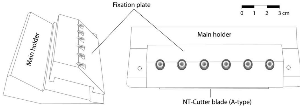
**Fig. 3.** Schematic view of the removable blade holder designed for the use of NT-Cutter blades. The base (main holder) is angled to guarantee an optimized basic angle of the removable blade relative to the sample surface.
