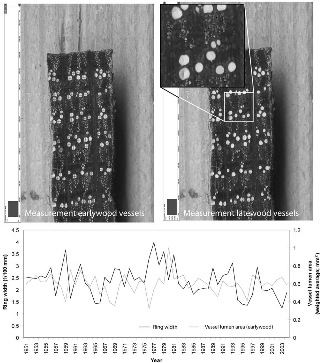
**Fig. 8.** Example for an automated measurement of earlywood (upper left) and latewood vessels (upper right) based on the scan image of a *Quercus petraea* core (compare Fig. 7). The lower diagram illustrates the resulting mean earlywood vessel size variation along the entire core as well as the respective ring-width variations.
