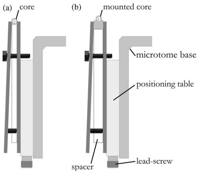
**Fig. 2.** Schematic (side) view of the sample holder (compare Fig. 1) illustrating the fixation of (a) unmounted and (b) mounted cores by using different sized spacers. The height and the thickness of the spacer for mounted cores depend on the size of the mount.
