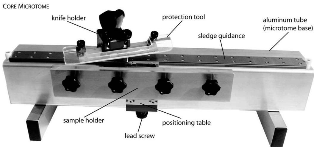
**Fig. 1.** . The core-microtome and its components as described in the text. The protection tool is designed to be placed on the microtome knife to avoid injuries while handling the microtome.
