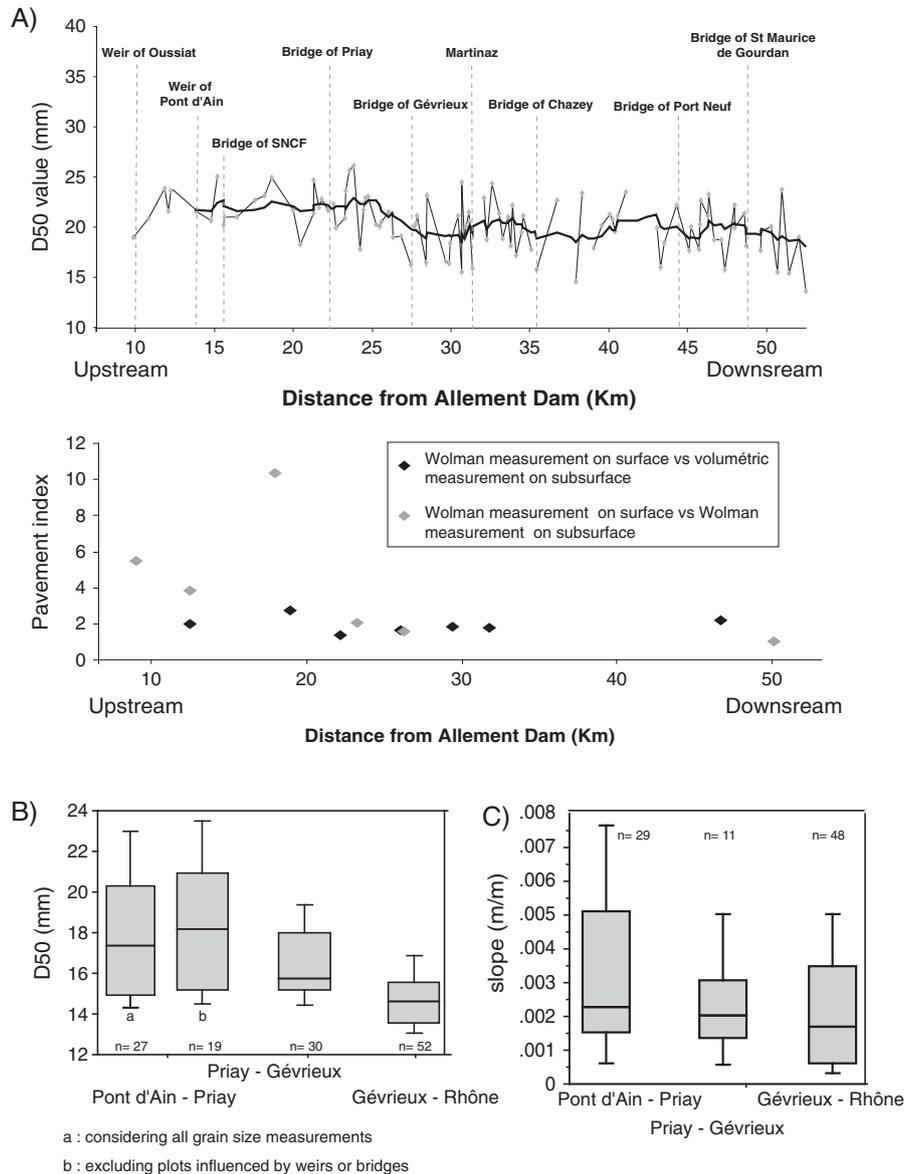
Figure 4. (A) Longitudinal distribution of grain size (dark line corresponds to the moving average of rank 5) and pavement index, (B) grain size distribution within the three studied subreaches (distinction is justified in the text) and (C) channel slope from Pont d'Ain to the Rhône River. Box plots provide a set of centile values, the 10th, 25th, 50th, 75th and 90th
