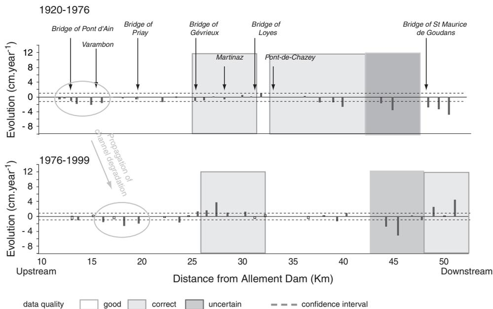
Figure 5. Longitudinal representation of the vertical evolution of the river bed between 1920 to 1976 and 1976 to 1999 ('Good', 'correct' and 'uncertain' refer to the data quality, see material and method for details)
