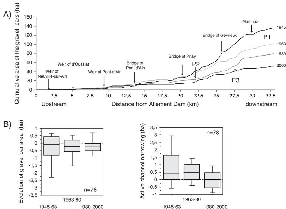
Figure 3. (A) Cumulative gravel bar areas in the active channel in 1945, 1963, 1980 and 2000 from Allement Dam to Chazey (measured per unit reach of 250 m long) and (B) evolution of gravel bars areas and active channel narrowing from 1945 and 2000. Box plot provide a set of centiles values, the 10th, 25th, 50th, 75th and 90th
