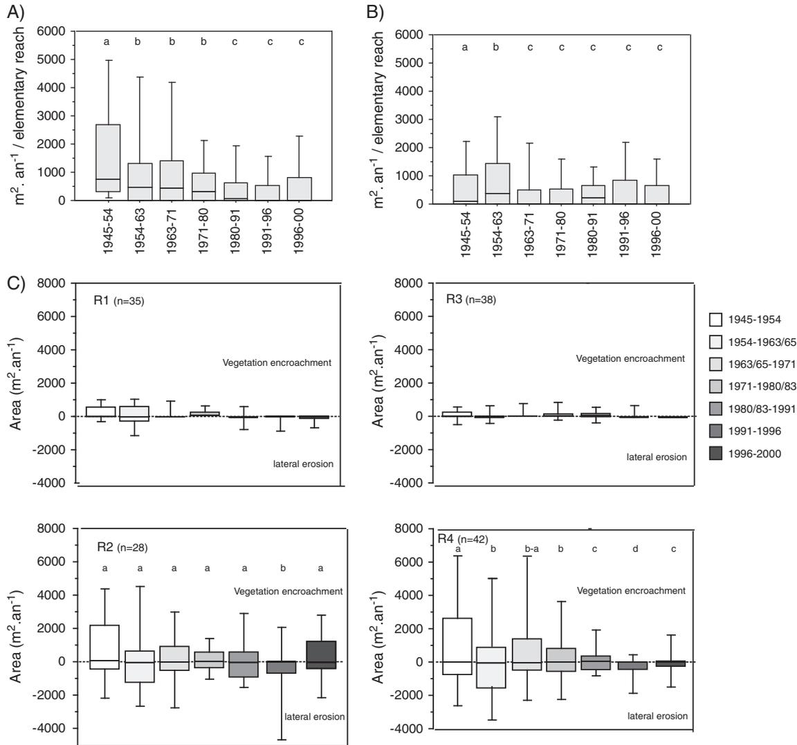
Figure 6. (A) Active channel narrowing, (B) mean floodplain area eroded between 1945 and 2000 (measured per unit reach of 250 m long,  $n = 144$ ) and (C) mean floodplain area vegetated and eroded per reach between 1945 and 2000 (R1 to R4 are reaches located in Figure 1.). Letters (a, b, c and d) indicate homogeneous groups (Wilcoxon test)
