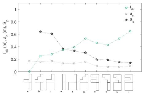
Fig. 6: Skier crack length, critical crack length and skier propagation index as a function of the profile type sorted to obtain a decreasing trend of  $S_n$ .
