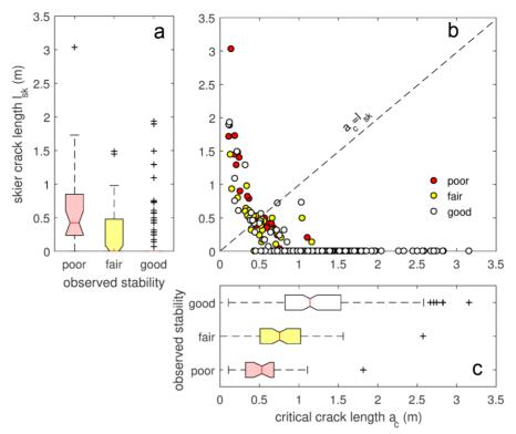
Fig. 7: Scatter plot and boxplots of the observed stability (based on RB scores) vs critical crack length  $a_c$  and skier crack length  $I_{sk}$  for R=3900 N.
