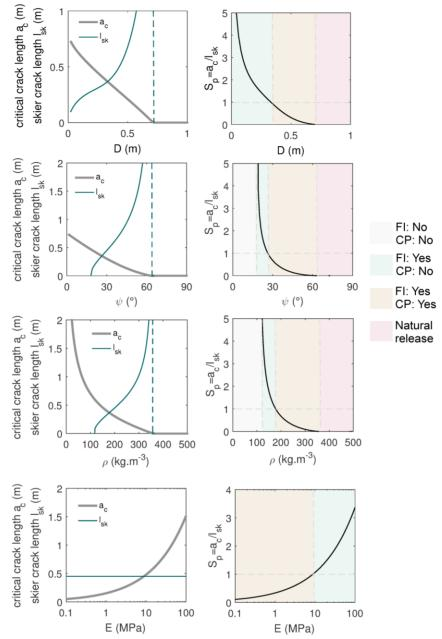
Fig. 4: Sensitivity analysis with independent snowpack properties, i.e. only one parameter was varied while the other properties were kept constant. D=0.4 m,  $\psi = 30^{\circ}$ ,  $\rho$ =200 kg m<sup>-3</sup>,  $\tau_p = 700$  Pa, R=780 N. FI: Failure initiation; CP: Crack propagation.
