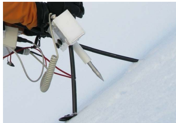
Figure 2: The snow micro-penetrometer (SMP) measures the penetration resistance of snow layers and due to its high resolution sensor allows the derivation micro-mechanical properties.
