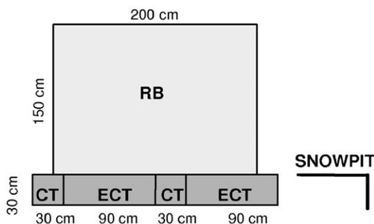
Fig. 1. Set-up for slope observations. Either one or two ECT and CT were done adjacent in front of the RB.
