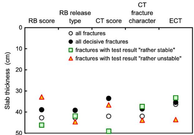
**Fig. 5.** Average slab thickness vs. stability test results for the RB, the CT and the ECT.
