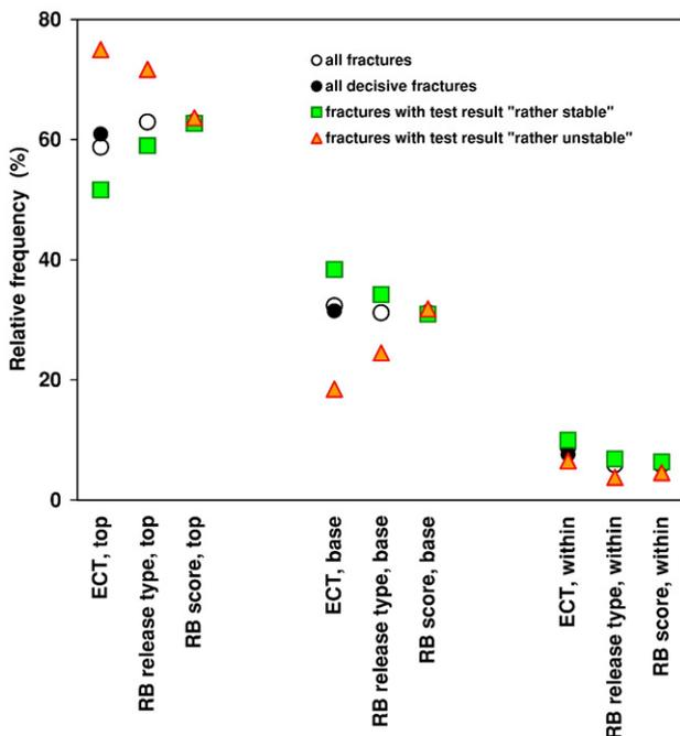
**Fig. 4.** Location and its frequency of the fracture in the failure layer for the ECT, the RB release type and the RB score.
