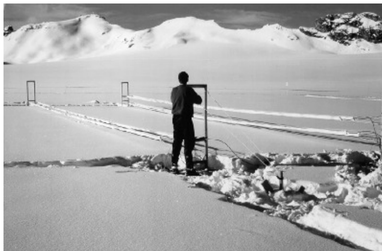
Fig. 8: Installation of the snow parameter measurement system on the glacier Plaine Morte. The site is located near Crans-Montana, Switzerland, at a height of about 2800 m above sea level and has favorable snow conditions even until June or July.
