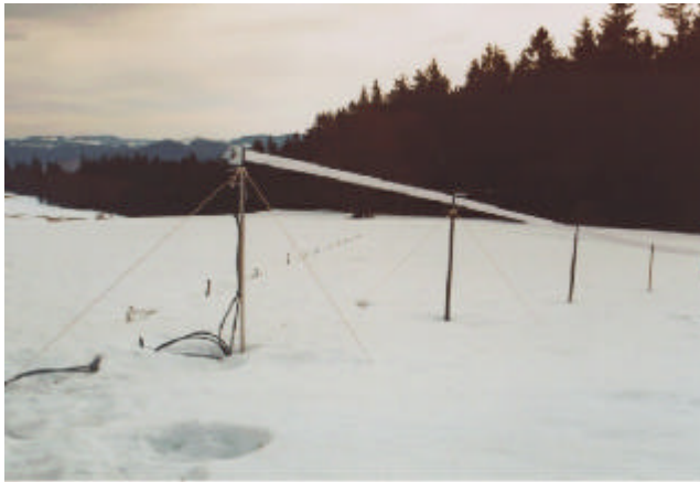
Fig. 14: Sloping cable for vertical profile measurements: installation and measurement results
