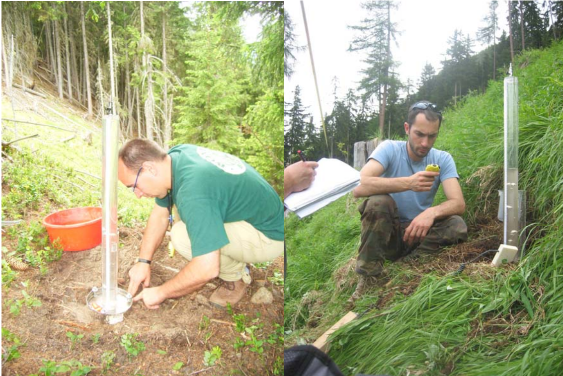
Figure 9: Experiments with infiltrometers to determine the infiltration rate. In the left picture, the water filled infiltrometer is connected to the soil (forest). At the right, the decrease of the water table in the infiltrometer is monitored (meadow).
