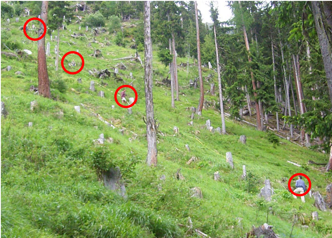
Figure 4: Preparation of the transect in the meadow to analyze the subsoil. The four collaborators (red circles) install the electrodes to measure electrical resistivity.
