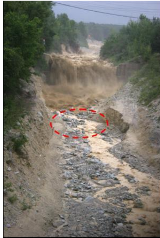
Arrival of the 1 July 2008 debris flow at the erosion sensor site (red ellipse; WSL, 1.7.2008)
