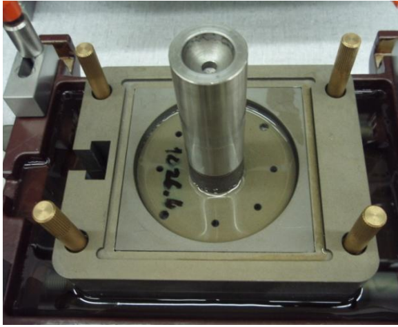
The shear box (10 cm x 10 cm x 2 cm) of IGT-ETHZ used for mechanical testing of the Rüdlingen soil.
