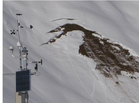
Automatic weather stations at the Wannengrat field site record meteorological parameters at 10 minute intervals. These data are used for a variety of research purposes, including avalanche formation.
