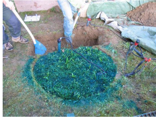
Dye tracer experiment to investigate water flow paths in the soil.
