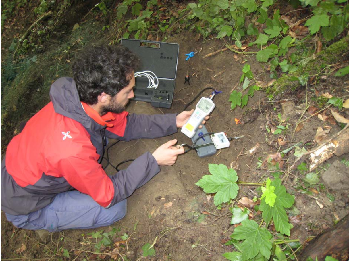
Fig.7 : pullout tests of roots.
