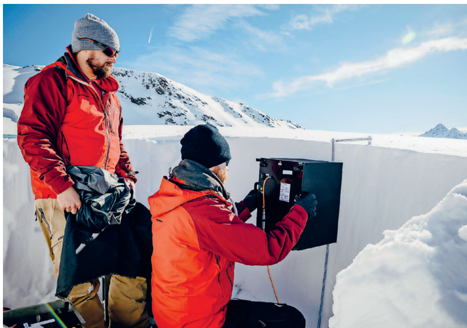
Taking measurements using infrared: the prototype of the SnowImager in action.
