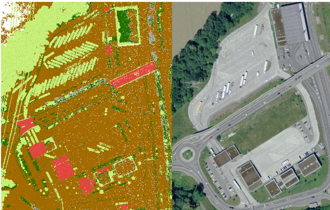
Figure 11: On the left picture, the LiDAR points classified by VVSC as low vegetation (light green), high vegetation (dark green) and buildings (red), and on the right an orthophoto of the area of interest that appears to be a parking, road and buildings.
