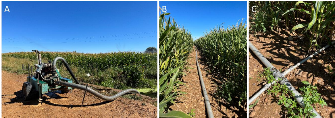
Figure 9: Aerial pipe irrigation infrastructure. From left to right: Engine pumping water out of ditch (A), aerial pipe transporting water to field (B), cross of aerial pipes with keys for different sections (C) (photos taken by Fabienne Frey in the area of SMI, 2022).
