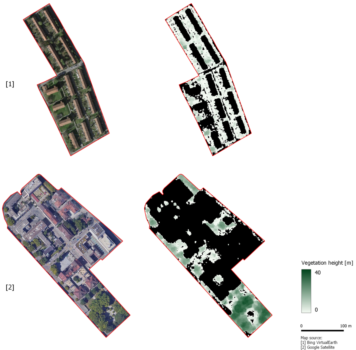
Figure 23: The super-/miniblocks with the highest [1] and the lowest [2] standard deviation in the vegetation height model. Both super-/miniblocks are shown with a satellite image (left) and the vegetation height model (right).
