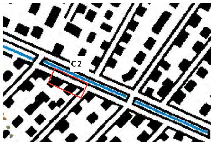
Fig. 18. Manual placement of sampling points on the 1:25000 topographic map. The point C2 was manually positioned at the intersection of two roads in order to be easily identifiable in the field.
