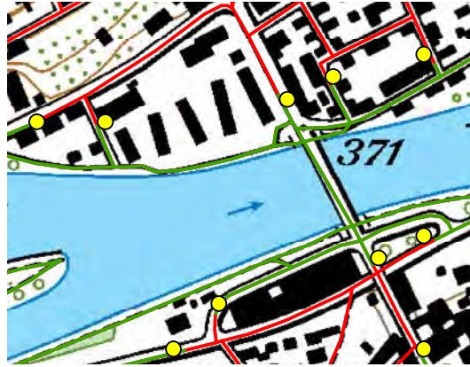
Fig. 7. Determination of river access points for pedestrians and cyclists. Access points (yellow circles) were obtained by intersecting roads situated along rivers (green lines) with roads not situated along rivers (red lines). Sources: © 2012 Swisstopo (Swiss street network), © 2102 Swisstopo (Topographical map).
