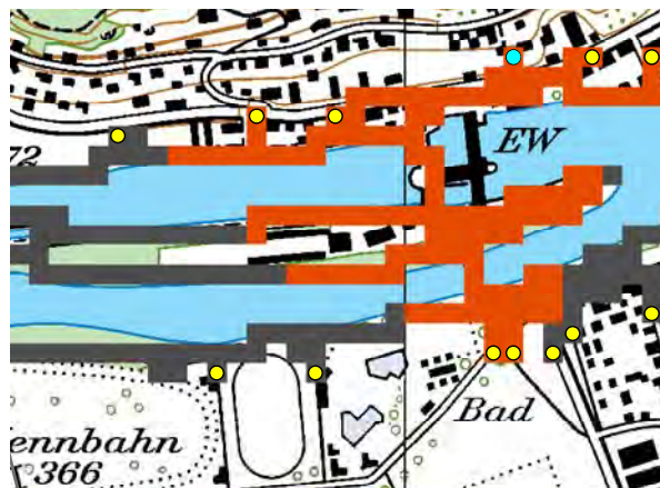
Fig. 13. Example of accessibility calculation for a given access point. Access points are displayed as yellow circles and the particular access point used in this example is displayed as a blue circle. The inaccessible stretches of the road network are displayed as grey lines while the accessible stretches are displayed as orange lines. In this example, a fake distance threshold of 500 m was used to illustrate the process. All orange stretches are accessible from the blue access point within a distance of 500 m and are assigned a value of 1, multiplied by the number of people present in the blue access point. Conversely, all grey stretches are assigned a value of 0 because they are not accessible from the blue access point. Sources: © 2012 Swisstopo (Topographical map).
