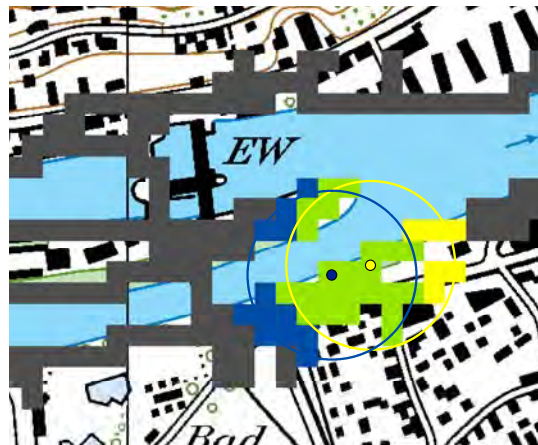
Fig. 15. Example of infrastructure score calculation. The blue dot represents a playground, while the yellow dot represents a picnic place. The perimeters of influence for both infrastructures are displayed as circles of a 100 m radius each, and of corresponding colours. All road raster cells falling within the perimeter of influence of the playground get a score of 0.4 and are displayed in blue, while all road raster cells falling within the perimeter of influence of the picnic place get a score of 0.45 and are displayed in yellow. Finally, road raster cells falling within both perimeters of influence get a score of 0.85 (equivalent to the sum of each of the respective weights) and are displayed in green, while all remaining raster cells get a score of 0 and are displayed in grey.
