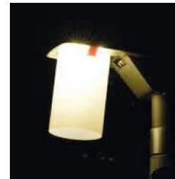
Figure 3: Diffusor mounted on streetlight (Picture: Martin Obrist, WSL).
