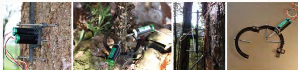
Figure M1 Collection of point dendrometers (natkon.ch). The carbon frames are either T-shaped (for large stems) or O-shaped (for small stems or branches) and are anchored in the stem with stainless steel rods. Up to three sensors are attached to the different type of frames in order to measure different expositions at the stem or to measure stem radius fluctuations over bark and on the xylem separately.
