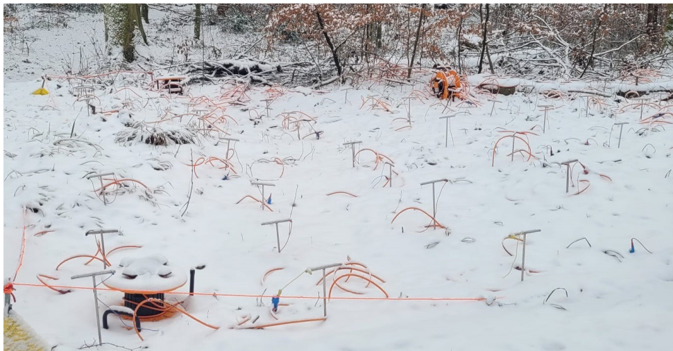
Above: A 3D survey carried out in Zurichberg in January to test remote monitoring.
