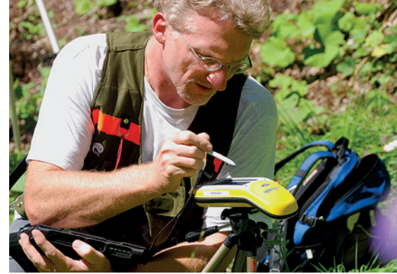
The centre of each sample plot is surveyed using terrain points and a GPS.
