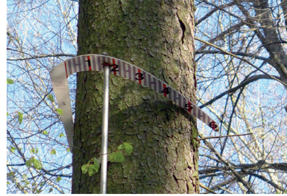
The diameter at a height of 7 m is measured with Finnish calipers.
