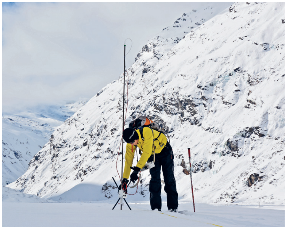
Researchers use the SnowMicroPen to measure the layers in the snow cover quickly and accurately.
