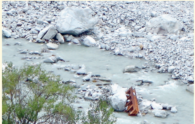
A debris flow swept away the three-ton set of scales in the Illgraben, depositing it in the Rhone river. In the photo you can see the large boulders that caused the destruction.
