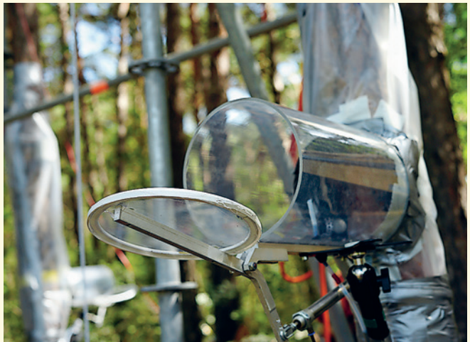
This is where the marked CO 2 respired by the enclosed tree collects.
