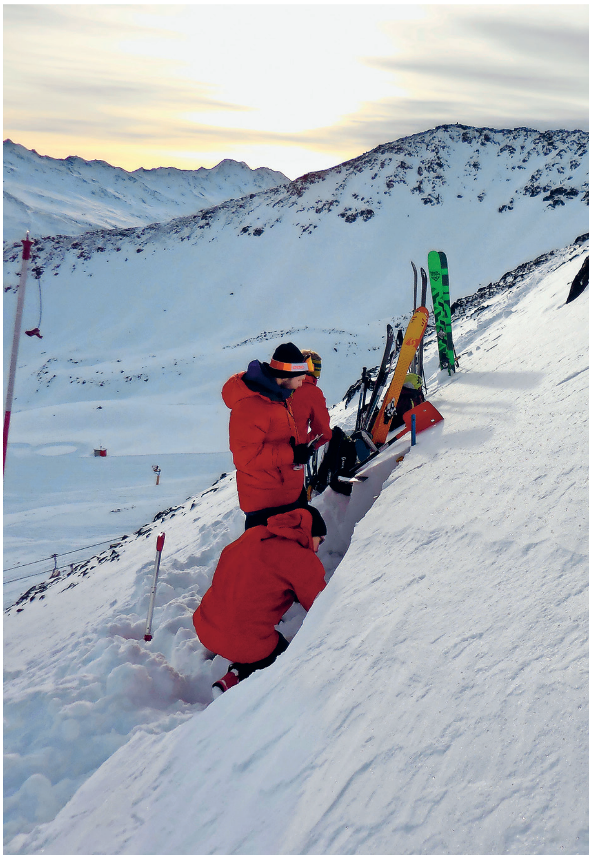
Field trip during a course: a snow profile provides information about the snow cover, which is important for assessing the avalanche danger.
