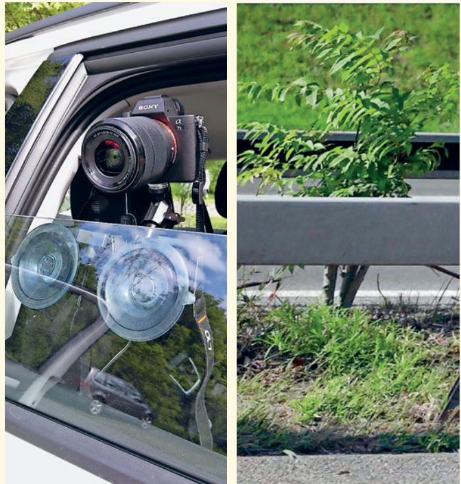
Cameras in the car film the vegetation on the left and right. The image of the tree of heaven (right), taken at a speed of 90 km/h, is astonishingly clear.
