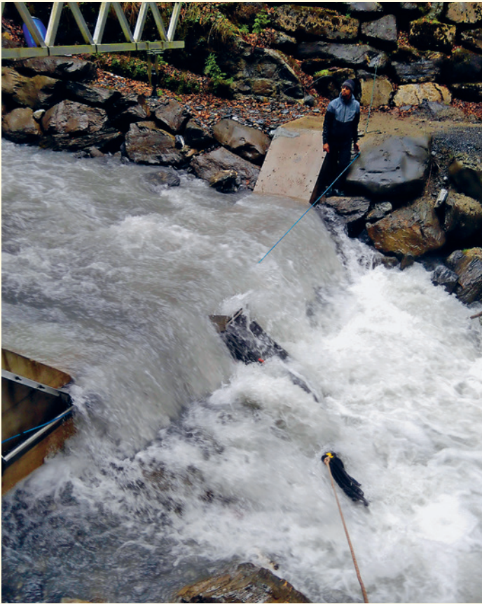
Researchers collect bedload with a net in the mountain torrent Avançon de Nant in Canton Vaud.
