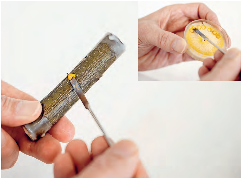
A spatula tip of fungal culture, taken from the Petri dish, is enough to infect the wood. Such infection experiments show how badly a pathogen affects a tree.
