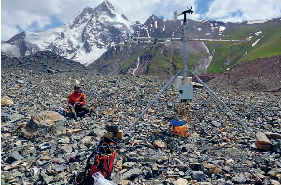
Testing an automatic weather station on the Kyzylsu glacier in Tajikistan. The glacier’s ice is hidden under a fifteen-centimetre-thick layer of debris.
