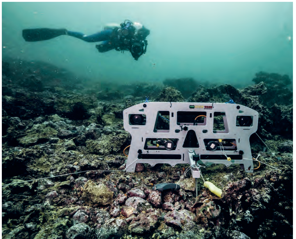
This device on the seabed makes video recordings of the species swimming past – here of a diver taking part in the expedition.
