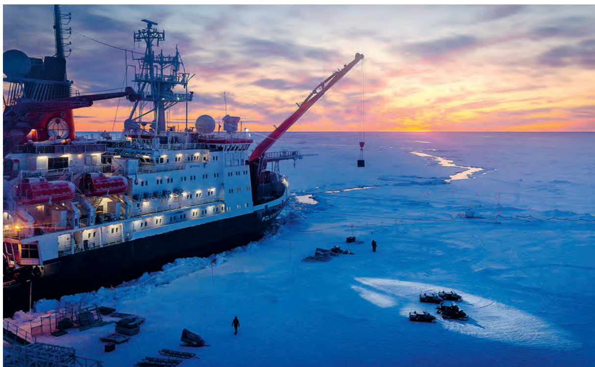
Even while the research ship was trapped in the ice, its engines had to be kept running constantly – for heating, light and cooking, as well as for operating the scientific measuring instruments.
