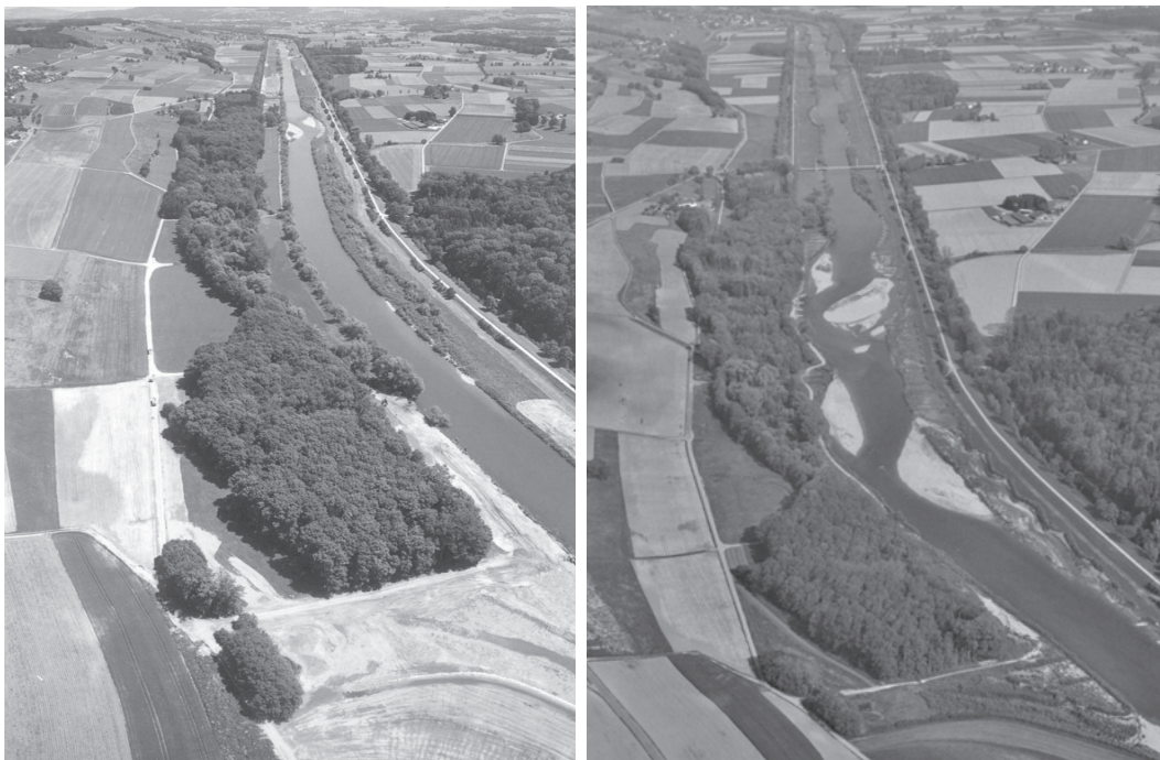
Figure 4.8: The Thur at Niederneunforn. Left: channelled Thur in June 2001. Right: revitalised Thur with alternating gravel banks (May 2004). (C. Herrmann, BHA team, Frauenfeld)
